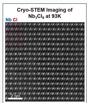
Cryo-STEM provides a direct probe of a new range of electronic phases
