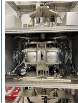
Fig. 8: Internals of Laser Dode Floating Zone Furnace.
