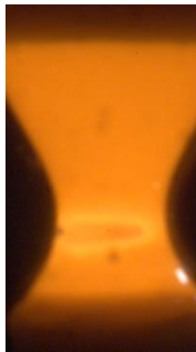
Fig. 2: Molten zone during growth in High Pressure Floating Zone Furnace.
